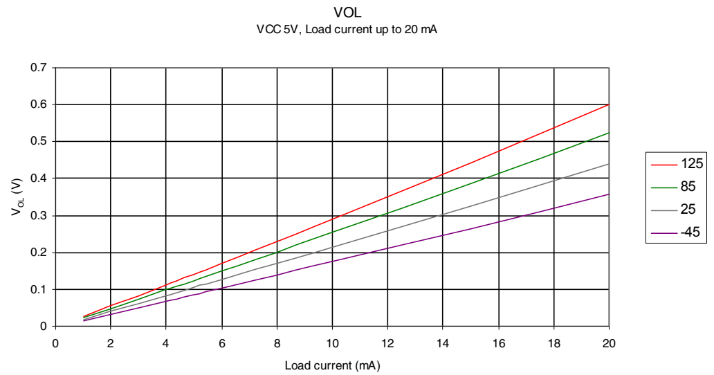
Figure 27-17. I/O Pin Output Voltage vs. Sink Current ( V_{CC} = 5V )
