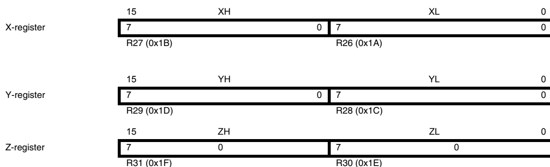
Figure 12-3. The X-, Y-, and Z-registers
