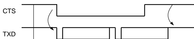
Figure 25-28. Transmitter Behavior when Operating with Hardware Handshaking
