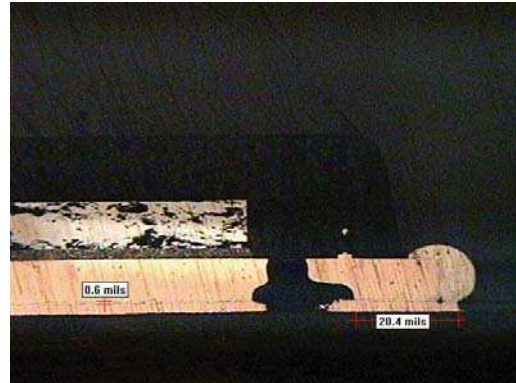
37% Paste coverage, Encroached Via, 0.6 mil Standoff
