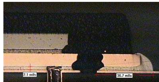
81% Paste Coverage, Encroached Via, 2.1 mil Standoff
