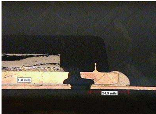
37% Paste Coverage, Plugged Via, 1.4 mil Standoff
