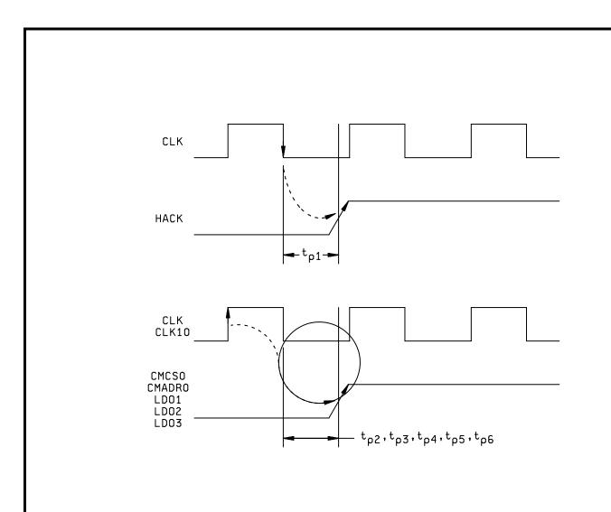
FIGURE 4. Timing waveforms.
