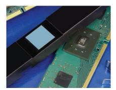
Hi-Flow 565UT is a naturally tacky, thermally conductive phase change material which is supplied in an easy to use tabulated pad form. In the application the material undergoes a phase change softening, starting near 52°C. The phase change softening feature improves handling characteristics prior to assembly. At application temperatures and pressures, Hi-Flow 565UT wets out the thermal interfaces resulting in a very low thermal impedance.
