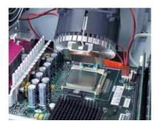
Hi-Row 225U is designed for use as a thermal interface material between a computer processor and a heat sink. The product consists of a thermally conductive 55℃ phase change compound coated on a release liner and supplied on a carrier.
