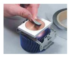
Bergquist reworkable Hi-Row 225FT thermal interface material provides a low thermal resistance path between hot components such as high performance processors and heat sinks. The material consists of a 55°C phase change compound bonded to one side of a conformable metal foil. This pressure sensitive material is easily applied to the heat sink and securely conforms to many mounting surfaces. Its compliant foil allows for easy release and reworking without leaving residue on CPU surfaces.
