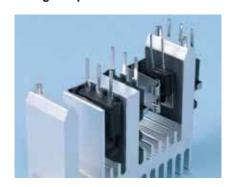
Hi-Flow 225F-AC is a high performance, thermal interface material for use between a computer processor and a heat sink Hi-Flow 225F-AC consists of a soft, thermally conductive 55°C phase change compound coated to the top surface of an aluminum carrier with a soft, thermally conductive adhesive compound coated to the bottom surface to improve adhesion to the heat sink.
