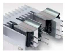
Bergquist Hi-Flow II5-AC is a thermally conductive fiber reinforced phase change material. The product consists of a thermally conductive 65°C phase change compound coated on a fiberglass web, and an adhesive coating on one side for attachment to a cold heat sink. There is no need to preheat the heat sink to apply the Hi-Flow II5-AC.
