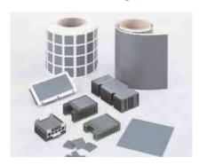
Hi-How 105 is a phase change material coated on both sides of an aluminum substrate. It is designed specifically to replace grease as a thermal interface, eliminating the mess, contamination and difficult handling associated with grease. Hi-How 105 is tack-free and scratch resistant at room temperature and does not require a protective liner in shipment when attached to a heat sink.
