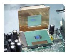
Bergquist's reworkable Hi-Row 225UF thermal interface material provides a low thermal resistance path between hot components such as high-performance processors and heat sinks
