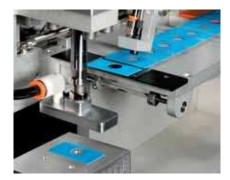
Bergquist SI-Pad 1500ST (Soft Tack) is a fiberglass reinforced thermal interface material that is naturally tacky on both sides SI-Pad 1500ST exhibits superior thermal performance when compared to the competitors' thermal interface materials SI-Pad 1500ST is supplied in sheet or roll form for exceptional auto-dispensing and auto-placement in high volume assemblies SI-Pad 1500ST is intended for placement between an electronic power device and its heat sink.
