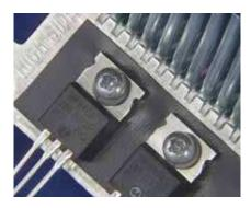
Sil-Pad 1200 is a silicone based, fiberglassreinforced thermal interface material featuring a smooth, highly compliant surface. The material features a non-tacky surface for efficient re-positioning and ease of use, as well as an optional adhesive coating. Sil-Pad 1200 exhibits exceptional thermal performance at low and high application pressures. The material is ideal for placement between electronic power devices and a heatsink for screw and clip mounted applications.
