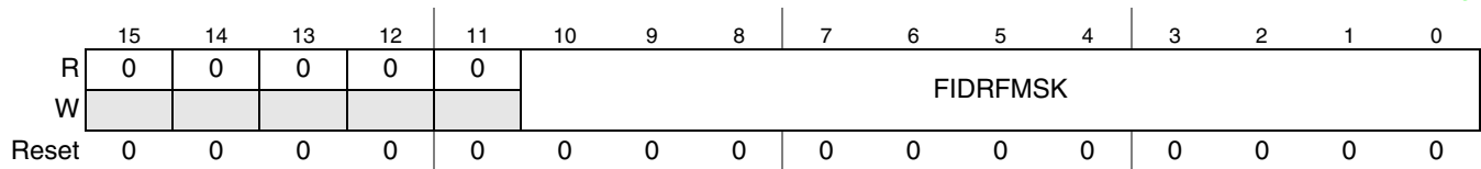
Figure 3-57. Receive FIFO Frame ID Rejection Filter Mask Register (RFFIDRFMR)
