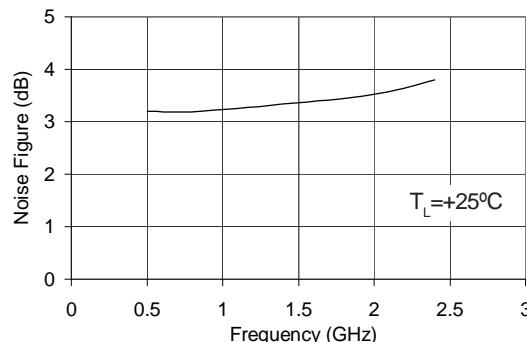
Typical RF Performance Over Temperature (Bias:  $V_D = 2.2\text{V}$ ,  $I_D = 20\text{mA}$  (Typ.))
