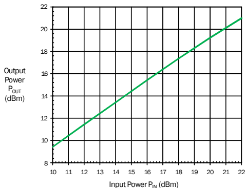
Output Power versus Input Power (Temperature=25°C, Frequency=1880MHz, VRF=1.8V)
