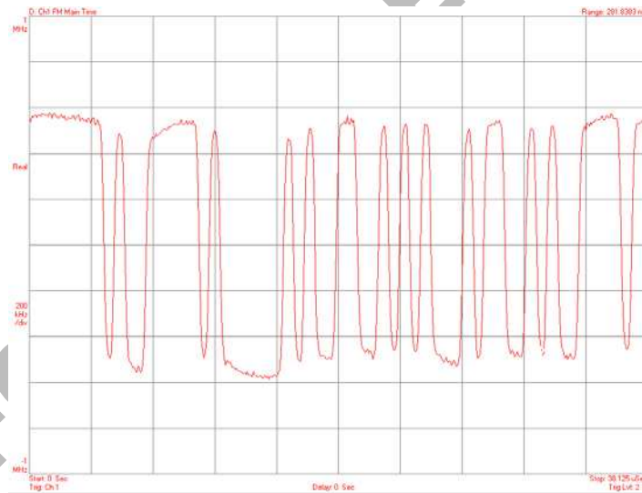
Figure 14 Measured frequency deviation in the time domain for 1.536Mbps, PN20 digital mode.
