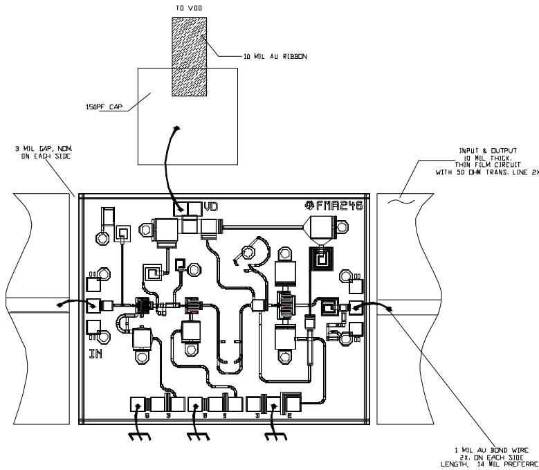
Note: <sup>1</sup>The supply de-coupling capacitor (150 pF recommended value) should be placed as close to the MMIC as practical.
