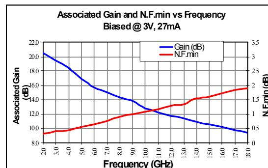
Noise Parameters (Biased at  $V_{DS}=3.0V$ ,  $I_{DS}=27mA$ )
