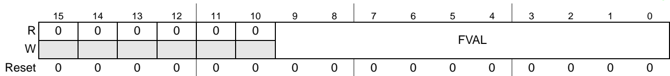
Figure 3-32. Sync Frame ID Acceptance Filter Value Register (SFIDAFVR)
