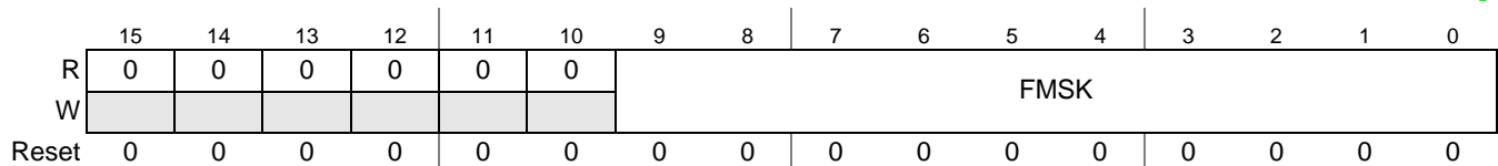
Figure 3-33. Sync Frame ID Acceptance Filter Mask Register (SFIDAFMR)
