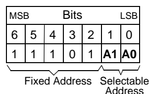
Figure 21. Address Bit Definition for 7-Bit Address
