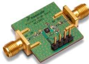
Figure 12. Typical Assembled Evaluation Board with SMA Connectors
