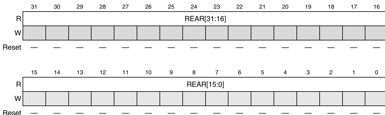
Figure 13-31. RAM ECC Address (REAR) Register
