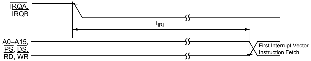
Figure 3-17 Interrupt from Wait State Timing
