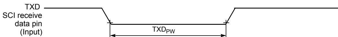
Figure 3-29 TXD Pulse Width
