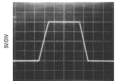
Large Signal Transient Response, V_S = \pm 15\text{V}
