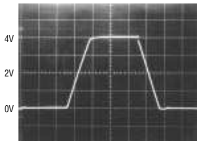
Large Signal Transient Response, V_S = 5\text{V}, 0\text{V}
