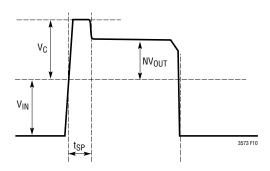
Figure 10. Typical Switch Node Waveform
