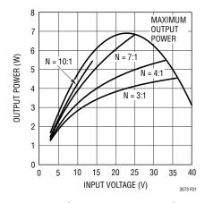
Figure 1. Output Power for 3.3V Output
