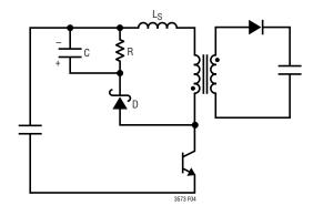
Figure 4. RCD Clamp
