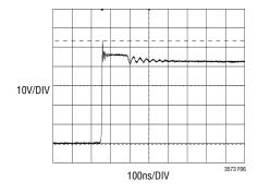
Figure 6. Good Snubber Diode Limits SW Pin Voltage
