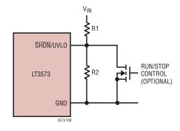
Figure 8. Undervoltage Lockout (UVLO)
