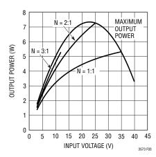
Figure 3. Output Power for 12V Output
