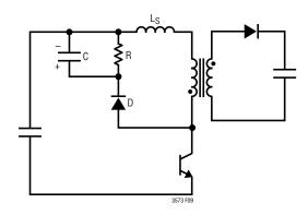
Figure 9. RCD Snubber in a Flyback Converter
