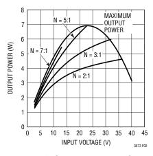
Figure 2. Output Power for 5V Output
