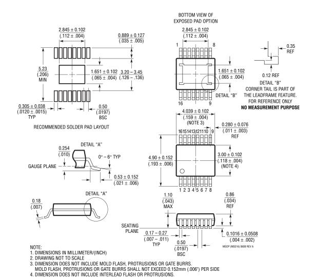
INTERLEAD FLASH OR PROTRUSIONS SHALL NOT EXCEED 0.152mm (.006") PER SIDE 5. LEAD COPLANARITY (BOTTOM OF LEADS AFTER FORMING) SHALL BE 0.102mm (.004") MAX
