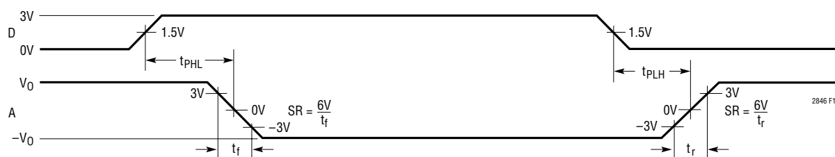
Figure 15. V.28 Driver Propagation Delays
