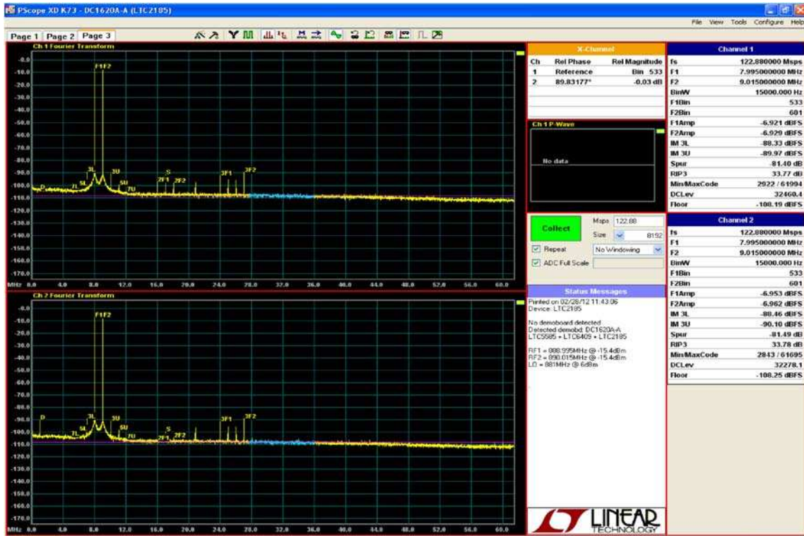
Figure 36. f_{RF} = 889\text{MHz} and 890\text{MHz} 2-Tone Receiver Test, f_{LO} = 881\text{MHz} . Ch.1 Is the I Channel and Ch.2 Is the Q Channel. Tested without LNA
