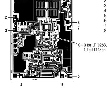
114mils × 81mils, Backside (substrate) metal: Alloyed gold layer Backside potential: Connect to V<sup>-</sup>
