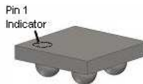
Figure 4. WLCSP Bumps Facing Down (Bottom View)
