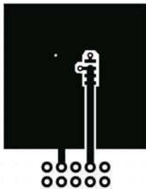
a) 50^\circ\text{C}/\text{W} when mounted on a 1 in 2 pad of 2 oz copper.
