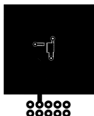
a. 65^\circ\text{C/W} when mounted on a 1\text{ in}^2 pad of 2 oz copper
