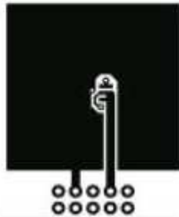
a. 78\text{ }^\circ\text{C/W} when mounted on a 1\text{ in}^2 pad of 2 oz copper
