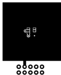
a) 130\text{ }^{\circ}\text{C/W} when mounted on a 1\text{ in}^2 pad of 2 oz copper
