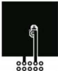
a. 78 °C/W when mounted on a 1 in 2 pad of 2 oz copper
