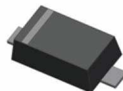
SOD-523F Band Indicates Cathode BAT54XV2 Marking : 5B
