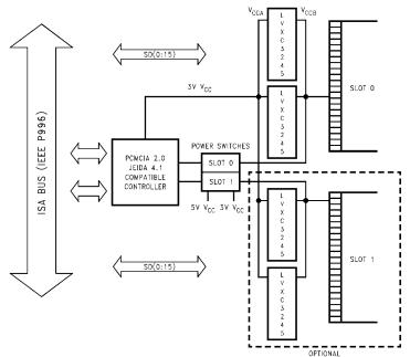
The LVXC3245 is a 24-pin dual supply device well suited for PCMCIA configurable I/O applications. Ideal for low power notebook designs, the LVXC3245 consumes less than 1 mW of quiescent power in all modes of operation. The LVXC3245 meets all PCMCIA I/O voltage requirements at 5V and 3.3V operation. By tying  $\rm V_{CCB}$  of the LVXC3245 to the card voltage supply, the PCMCIA card
