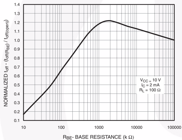
Fig. 9 Normalized t_{off} vs. R_{BE}
