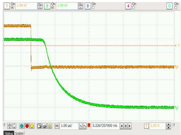
Figure 21. Turn-off Response ( V_{CC} = 3.3\text{ V} , V_{IN} = 5.0\text{ V} , R_L = 10\ \Omega , C_L = 0.1\ \mu\text{F} )
