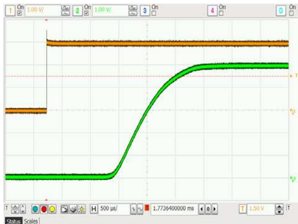
Figure 20. Turn-on Response ( V_{CC} = 3.3\text{ V} , V_{IN} = 5.0\text{ V} , R_L = 10\ \Omega , C_L = 0.1\ \mu\text{F} )
