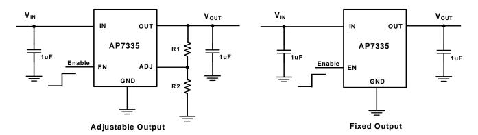
$$V_{OUT} = V_{REF} \left( 1 + \frac{R_1}{R_2} \right)$$
