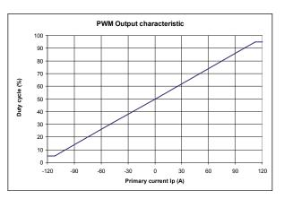
$$\begin{split} \textit{PWM period} \quad & T_{\textit{Period}} = T_{\textit{High}} + T_{\textit{Low}} \\ & \textit{PWM frequency} = \frac{1}{T_{\textit{Period}}} = 125\textit{Hz} \\ & \text{DutyCycle(\%)} = \frac{T_{\textit{High}}}{T_{\textit{Period}}} \times 100 \\ & \text{DutyCycle(\%)} = 50\% + \text{G} \times \text{I}_{\textit{P}} \text{ with G = Sensitivity (\%/A)} \end{split}$$
