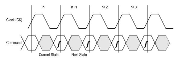
Current State and Next State Definition for: Pipeline and Flow Through Read Write Control State Diagram
