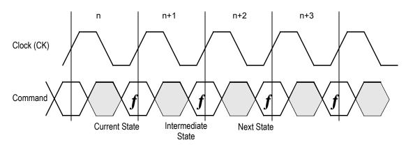
Current State and Next State Definition for Pipeline Mode Data I/O State Diagram
