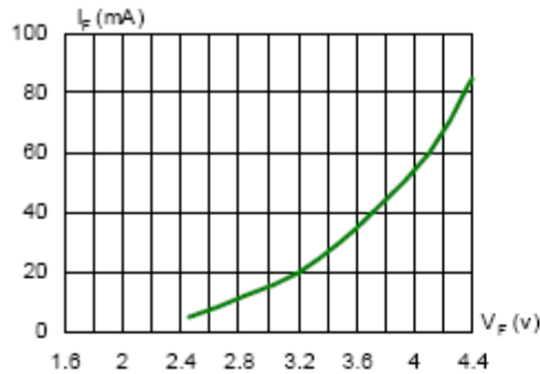
Fig.1 Forward Current vs. Forward Voltage
