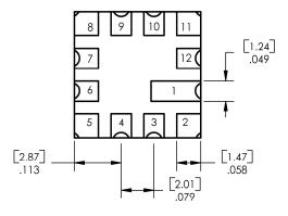
TOLERANCE IS ±.005 [ 0.13 ] DIMENSIONS ARE IN INCHES AND [MILLIMETERS].
