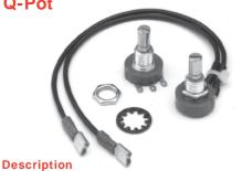
A high quality cermet potentiometer for use when linearity and stability are important and when high temperature or harsh environments exist. Accepts Versa-Knob or Lock Shaft. May be ordered with two 8 in. (20.3 cm) wires soldered to pot (clockwise increase) and female quick connect terminals on other ends by adding suffix X to end of part number.
