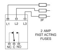
F = Fuses NO = Normally Open NC = Normally Closed C = Common, Transfer Contact
