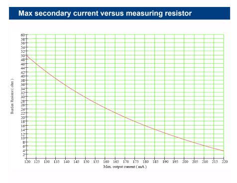
To maintain safe start-up  $\mathbf{R}_{M}$  must not exceed 2.5  $\Omega$  during fault condition.
