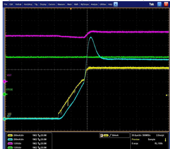
Figure 9. I_{VIN} , ILED Startup ( I_{LED\_OUT}=800mA )
